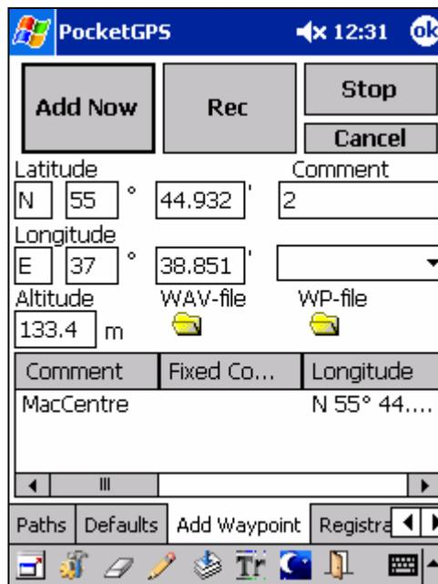
This dialogue is designed for fast addition of waypoints during movement. For convenience of using this dialogue, it is recommended to create an **Add Waypoint** button in one of fields in the main program window. It will allow to open this dialogue quickly. When opening the dialogue, data of the current user's location are displayed in edited fields.
