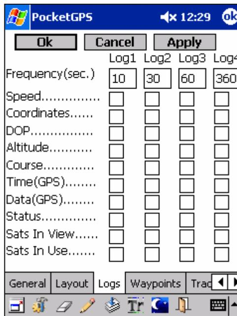
Using this dialogue, a user log can be customized. During a work, the PocketGPS can record the data about a location, speed, altitude, etc. in a log files. It is possible to specify, which data, and with what frequency, shall be written in these log files, and a quantity of log files (from 0 to 4).
