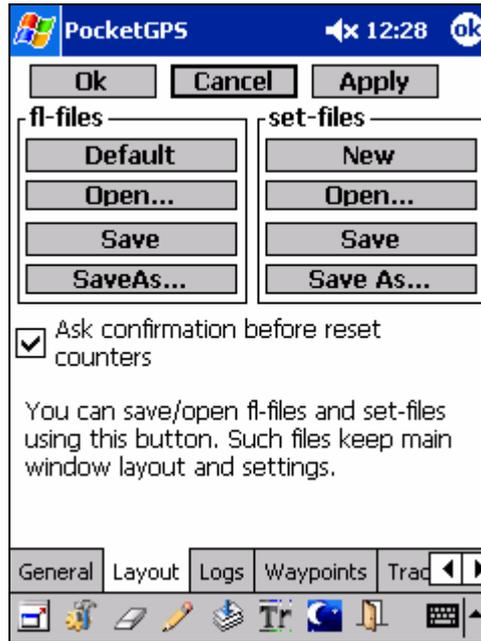
Using this dialogue box, it is possible to access the following functions: Create a new layout, Open a layout, Save, Save as... a current layout (.fl files) and current sets (.set files). In this dialogue box, a confirmation before reset of various counters can be requested, for example: the average speed counter.
