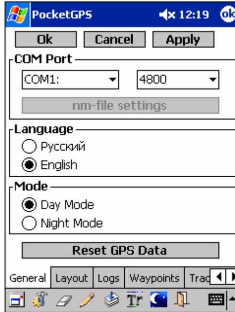
Using this tab, it is possible to specify, where the PocketGPS should take the data: from COM port (COM1-COM9) (i.e. directly from the GPS receiver) or from a previously written .nm file); language of the interface (Russian/English); night/day mode. The current GPS values can also be set to default (if GPS is connected, you will not see an effect from pressing this button, as the reset values will be replaced with current ones).
