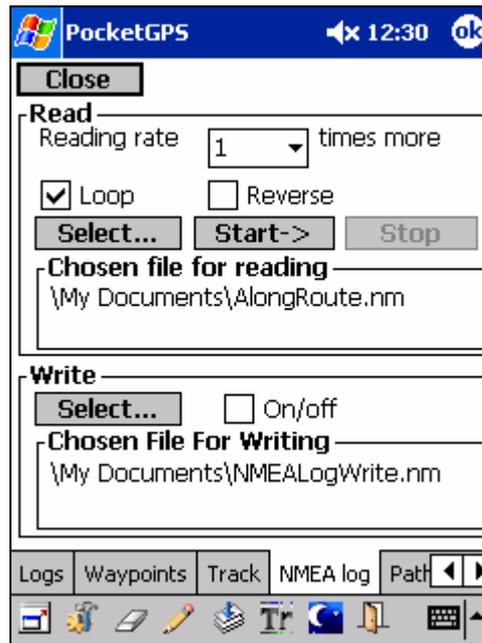
Using this dialogue, options connected with reading and writing the NMEA format data can be set.
